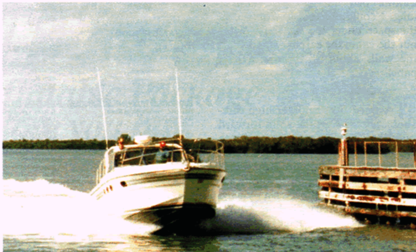
The advanced modified deep-V hull has a reverse sheer transom which extends planing length.
