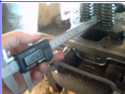
(4) Measuring the distance the injector control rod sticks out the back of the injector.
