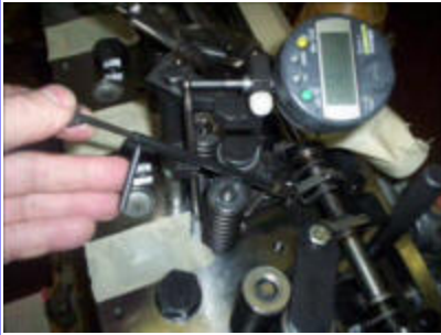
(2) John Whelan describes how to adjust the the injectors with the proper Caterpillar tools.
