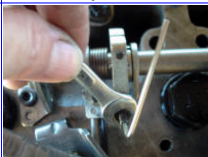
(6) Adjusting the CAT injector synchronization.
