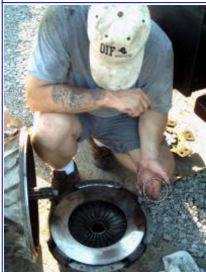
Trying to figure out how to get the retainer ring back on the throw out bearing.
