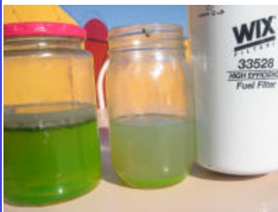
(3) Fuel Samples; Left is from the bottom of the fuel tank, and right is out of the fuel filter.
