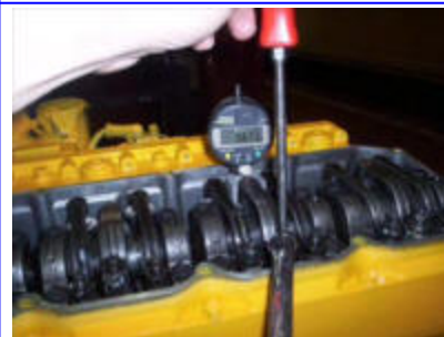
(3) John Whelan demonstrates adjusting the fuel injector rocker. Movie
