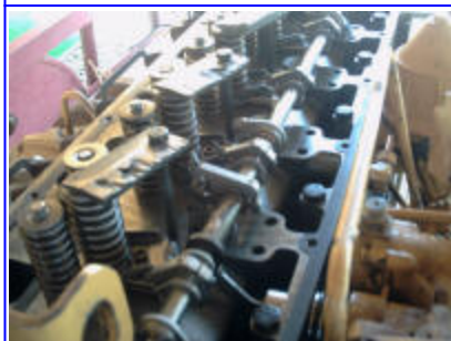
(3) Bits of steel using the rocker arm assembly bolts to slightly compress the injector springs.
