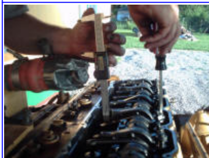
(7) Setting the injector timing is simply a matter of using a caliper to measure the height of the injector's spring.
