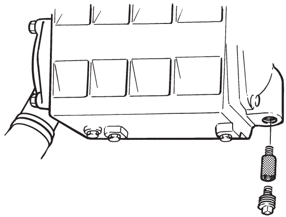
TAMD63, TAMD73 and TAMD74: Zinc anode in heat exchanger's front end cover
